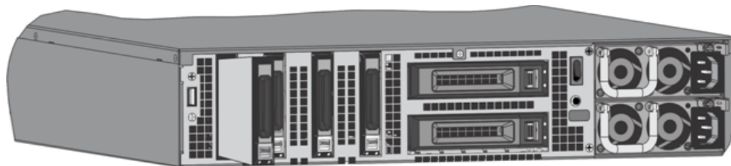
Figure 1-18. Inserting the Replacement Solid-State Drive
